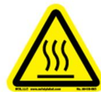
Burn Hazard / Hot Surface
